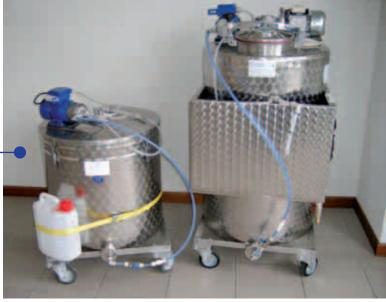
Internal tank 100-130-200-300 or 400 litres with double pump, double agitator, and sphere of washing (only over 200 lit). Easy transporting for making the washing operations at the farm.
